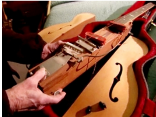
Solid-body “Log” guitar by Les Paul, made from a 4x4 wooden post to which a timber neck and pickups were attached. The curved sides were for appearance only.
